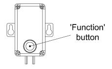
To enable the tap to be cleaned, a feature which blocks the water flow has been integrated. By pressing the function button the sensor is blocked for 30 seconds. The red light flashes (double flashes) during this period allowing cleaning without accidental operation.
